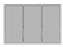
Figure 25 - Correct Burner Flame Pattern
